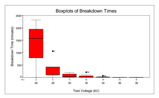
The positions of medians indicate that the median breakdown time decreases exponentially as the voltage level increases. The observations obtained by subjecting the fluid to the voltages of 36 and 38 kV exhibit very small spread making their boxplots flat.
