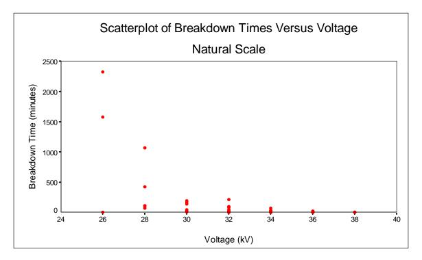
**4.3** SPSS can also be used to obtain a scatterplot of breakdown times versus voltage levels:
